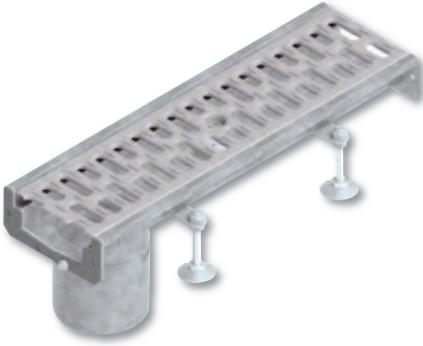
Shallow invert surface drainage system, manufactured from hot-dipped galvanised steel to BS EN ISO 1461:2009. Grating choice includes galvanised steel perforated, slotted and composite black and white to Load Class C250 to BS EN 1433. All gratings supplied complete with locking.
