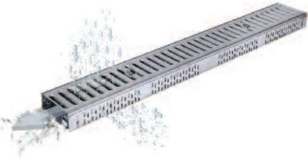
An advanced roof and balcony drainage system combining line drainage with point drainage by using an open sided drainage channel system to collect and convey rainwater to drainage points within a raised or suspended deck structure. Ideal for terraces, balconies, patios or roof gardens. FreeDeck allows free drainage through the channel wall with accessible outlets providing maintainability. Available in both galvanised and stainless steel.
