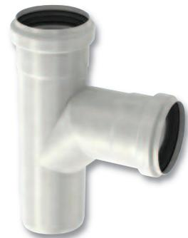
Wide range of socketed waste pipework systems in thin-wall stainless steel for above and below ground drainage applications. Manufactured from 304 and optional 316 grades stainless steel, ACO Pipe® provide the modern metal alternative to PVC-u and cast iron soil and waste pipework.
